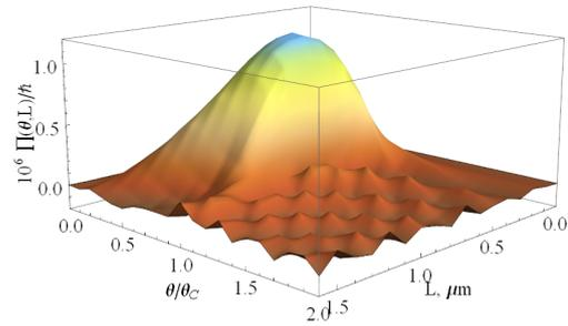
Figure 4. The SAM (6) of the radiation from 350 MeV positrons at (100) channeling Si as the function of angle of incidence and the crystal thickness.  $\theta_c$  is the critical Lindhard angle
