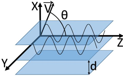
Figure 1. The scheme of orientation of the initial velocity of positrons in the system of crystallographic planes
