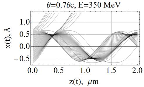
Figure 2. The 50 calculated trajectories of 350 MeV positrons at (100) channeling in Si crystal. The angle of incidence  $\theta$  is 0.7 of the Lindhard critical angle ( $264 \mu\text{rad}$ )
